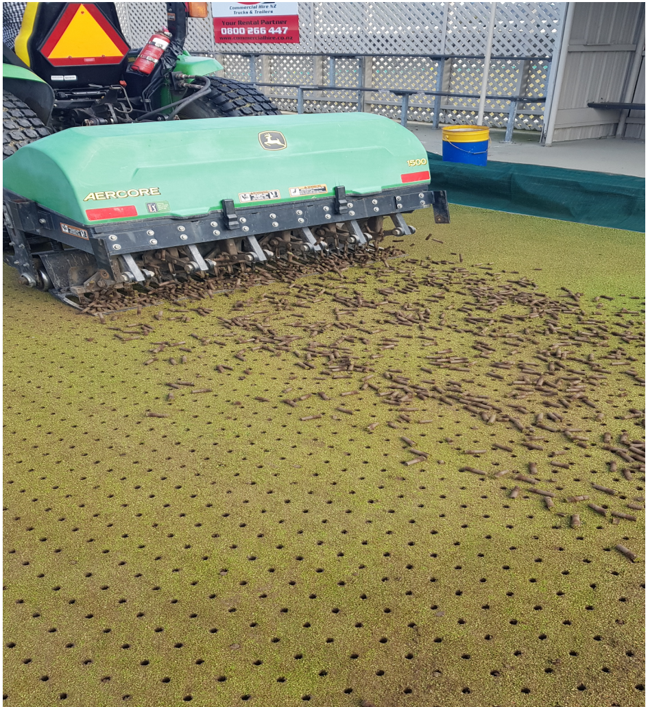
Coring Bowling Gren with Aercore machine 16mm dia. cores and back-filled with dry soil.
